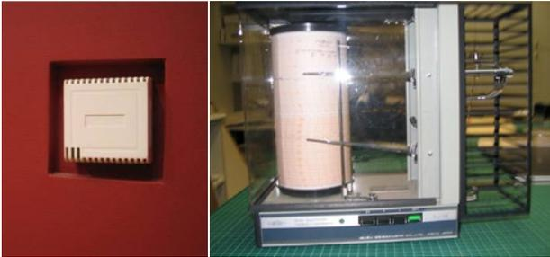
Images: Today's wall mounted thermohygrograph (left), and an older example (right), still used in some museums and galleries.
